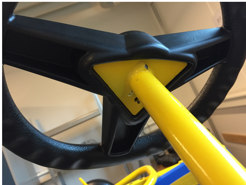
Figure 12. Another example of a poke-a-yoke solution. The steering wheel of a pedal car which can only be fastened in one way, thus always resulting in the correct alignment of the steering wheel.
