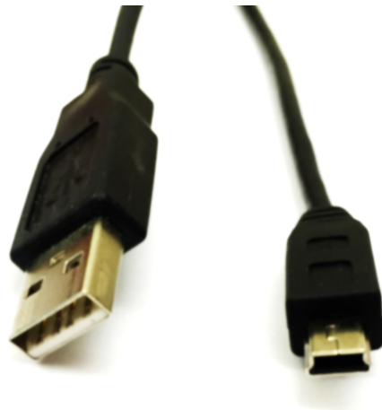
Figure 11. Example of a physical constraint where either ends of the USB cable has to be connected the right way.
